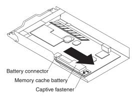
Figure 41. Removing the battery unit from the controller
